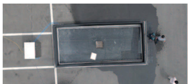
4. Fire release position fully submerged, battery stabilized
